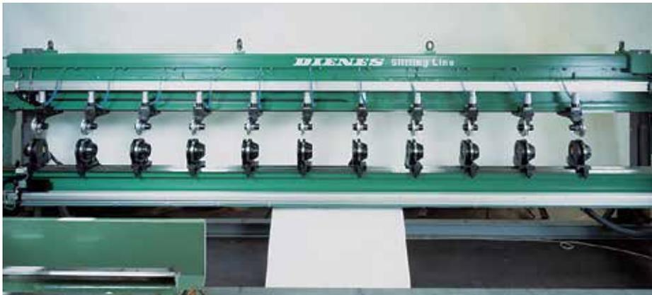
An example of a Jagenberg sheeter from 1977 shows how modernization results in significant cost savings. It was possible to reduce the setup times by more than 70% by means of installing a fully automatic slitting system.
