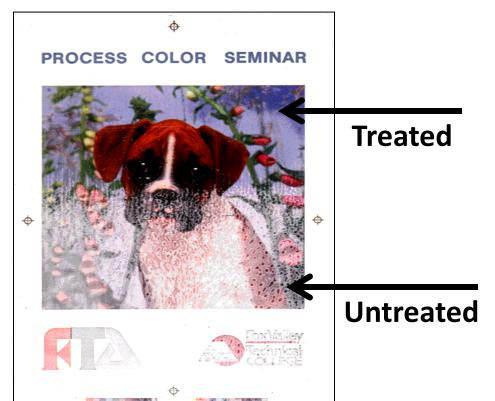
Prior to printing, the upper half of this film was corona treated while the bottom half was not.
