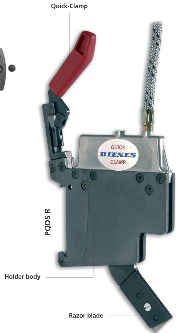
Razor blade head with adjustable engagement angle, which lengthens blade life.
