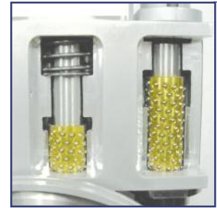
Ball-bearing knife holder axles
