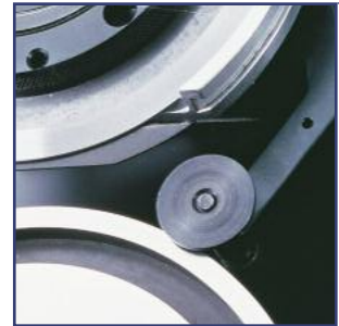
Adjustment slide Simple adjustment to bottom knife
